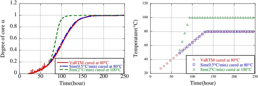
Figure 2: Experimental and simulated degree-of-cure curves and temperature of CFRP.
