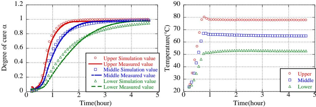
Figure 2: Degree-of-cure and temperature curves of the thick GFRP measured by multi-points measurement system.
