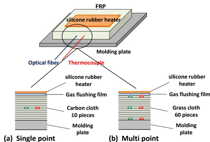
**Figure 1:** Experimental set-up and stacking configurations for cure monitoring of CFRP and GFRP.
